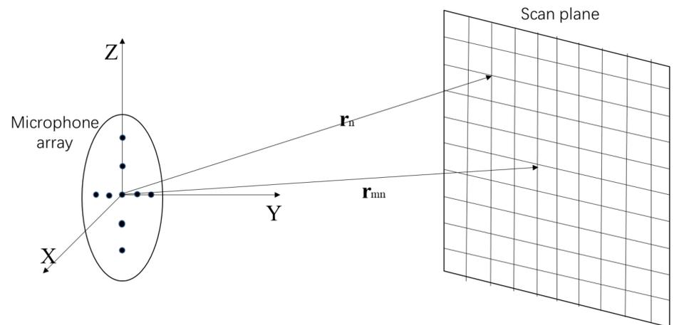
Fig. 1 Acoustic imaging detection model
